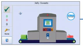
**Easy to Use Intuitive Full Colour Touchscreen** The X<sup>5</sup> Pack includes an Icon driven full colour touchscreen control interface including multilevel password access and data logged events for traceability (designed to comply with CFR21 Part 11 requirements)
